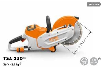
Easy-to-manoeuvre battery cut-off machine for 230 mm cutting wheels. Suitable for indoor and outdoor use, up to 70 mm cutting depth, water connection with ball valve and hose coupling for wet cutting, spindle lock, maintenance-free belt drive. For more information on features and technical details, see page 176.
